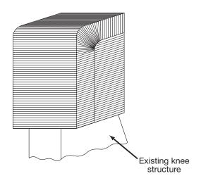
Covers top and one or both sides of knee structure — prevents damage during ship assist and empty barge service
