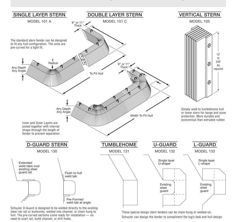
The stern fenders are custom built of durable, nylon reinforced, synthetic rubber. The rubber laminates are compressed onto high quality steel rods welded or attached to end plates. The steel rod and plate frame is allowed to flex through the use of a patented hinge type assembly system. Chain links are installed top and bottom as specified, and the end plates can be flat or angle. Our fenders are manufactured for a tight hull fit. These models are also available with weld tabs.
